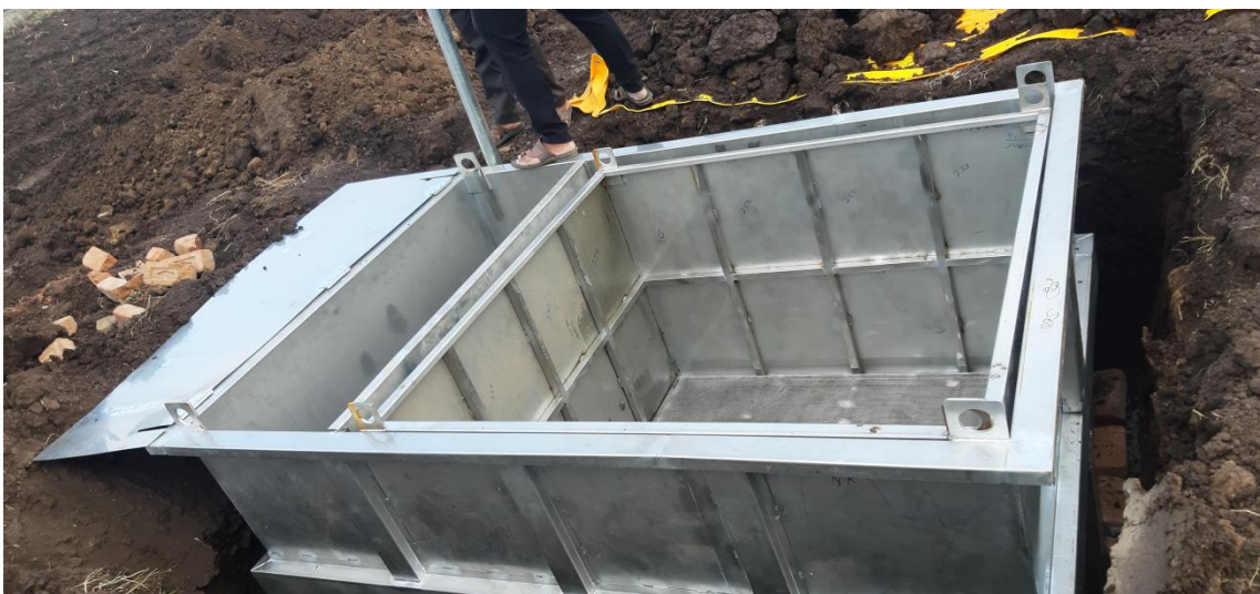
Fig. 9. Lysimeter placed on the foundation in pit
