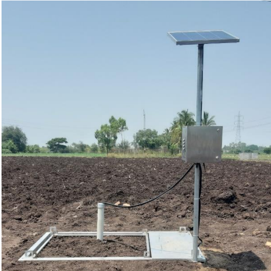
Fig. 14. Final installation of lysimeter and control panel
